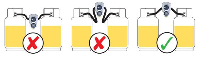
Always install the changeover regulator above the cylinders. This ensures that your Clesse regulator does not fill with condensed LPG product, giving longer service life.
