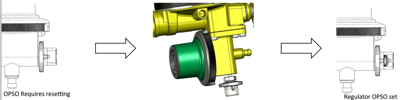
1. Over Pressure Shut Off must be reset by a qualified gas engineer, who should establish any cause for tripping, particularly if this device trips repeatedly.
