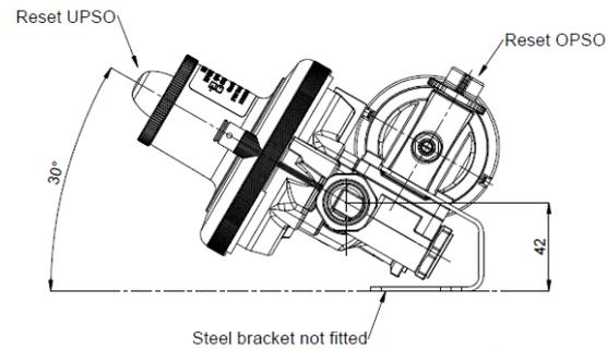
The wall bracket is set for 32mm riser, but is adjustable to accept 25mm and some variability. It can be shaped to meet contour of the wall.
