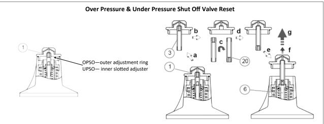
Fine adjustment of the OPSO setting is preformed beneath the OPSO vented cap 1 - both UPSO and OPSO are adjusted here. The outer ring adjustment is OPSO and the inner slotted adjuster is UPSO. Do not set pressures above the maximum limit of OPSO spring and take due care to the constraints of downstream pipework and equipment.
