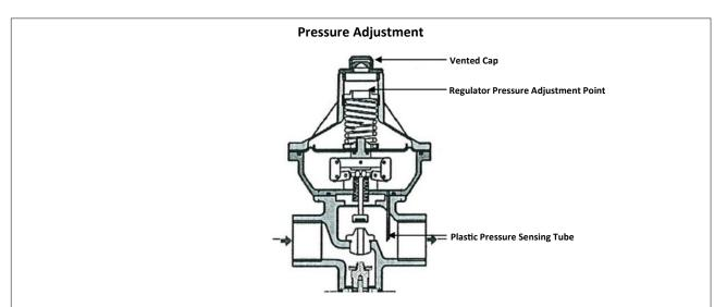
Fine adjustment of the regulator is performed beneath the main diaphragm vented cap (a 27mm socket is required). Do not set the pressure above the maximum limit of the regulator spring and take due care to the constraints of downstream pipework equipment.
